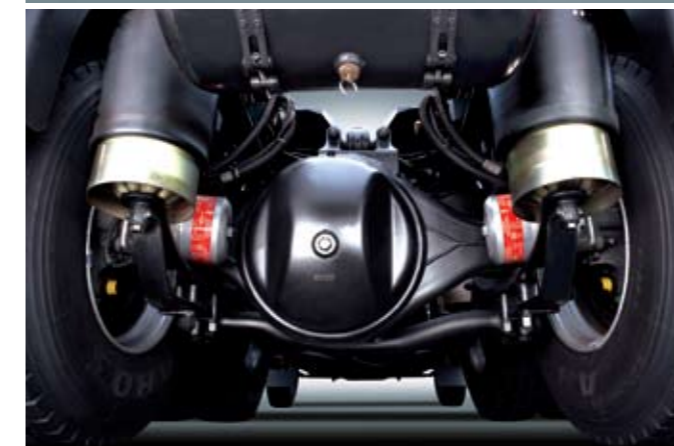
Automatic (ECAS) 4-bag type air-suspension
