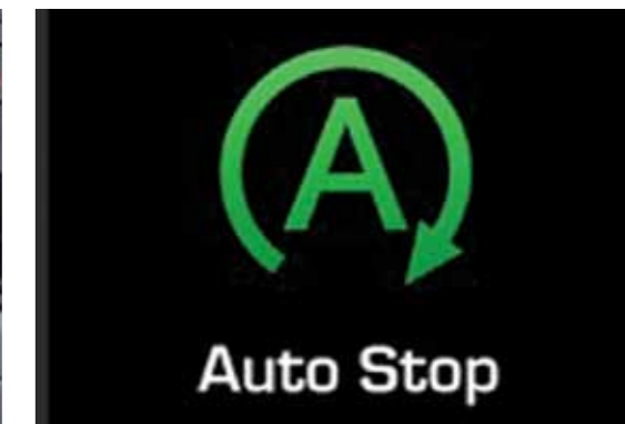
Idle Stop & Go (ISG) avoids unnecessary engine idling when stationary
