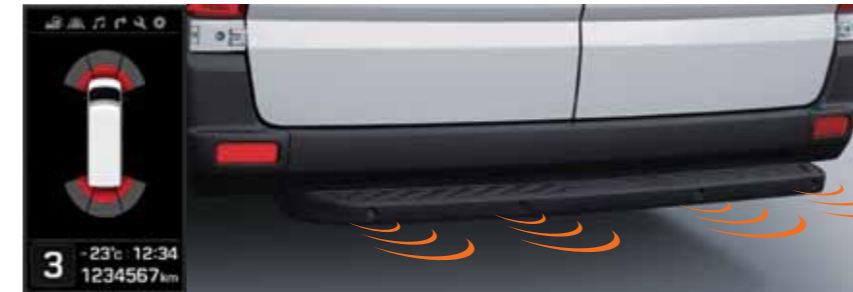
Park Assist System (PAS) uses strategically positioned sensors, front and rear, to detect potential obstructions when parking
