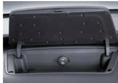
Storage tray with 12V power outlet. Located centrally on the upper dashboard
