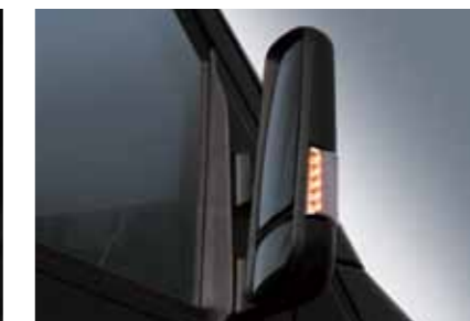
LED side repeater turn signals located in door mirrors
