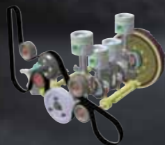
Long-life chain-drive for camshafts
