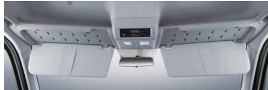
Sun visors, with integrated ticket holders, fit neatly into the roof shelf
