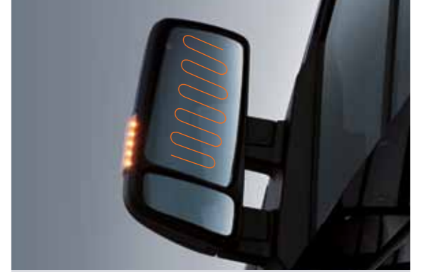
Side mirrors are electrically adjusted and heated
