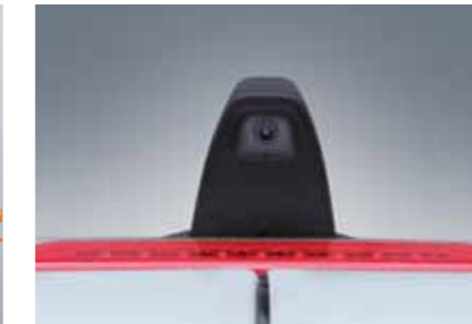
Rear camera feeds visual information to the in-cab display
