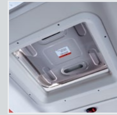
Natural Type Ventilator The manually operated roof hatches ventilate the passenger compartment which give the passenger can enjoy outside fresh air so easy.
